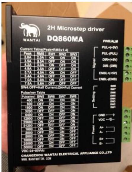
Fig.6: motor driver in use for lab prototype
